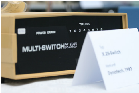
Abb. 16 Switch / Multi-Switch X.25
