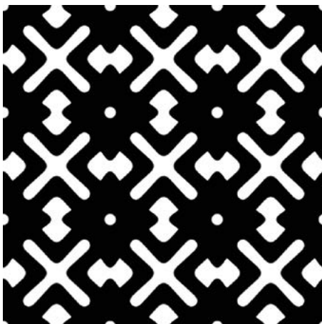
A periodic base cell exhibiting a large phononic band gap is shown tiled 3x3.
